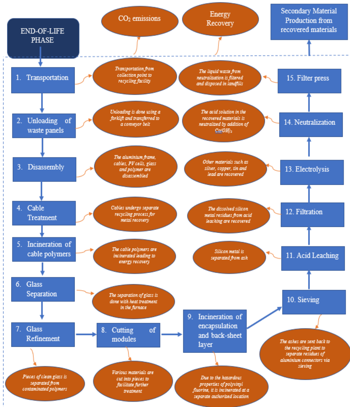
Figure 3.6: Steps in c-Si PV module waste treatment based on FRELMP method
