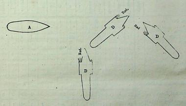
If A sees a White Mast-head Light above the Red Light, A knows that the vessel is a steam vessel, and is either approaching her in the same direction, as B, or is crossing to port in some direction, as D D D.
