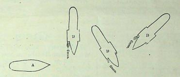
If A sees a White Mast-head Light above the Green Light, A knows that the vessel is a steam vessel, and is either approaching her in the same direction as B, or is crossing to starboard in some direction, as DDD.
