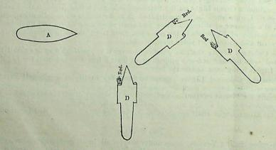
If A sees a White Mast-head Light above the Red Light, A knows that the vessel is a steam vessel, and is either approaching her in the same direction, as B, or is crossing to port in some direction, as D D D.
