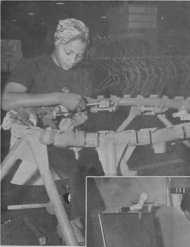
Assembling a bomber motor mount.
