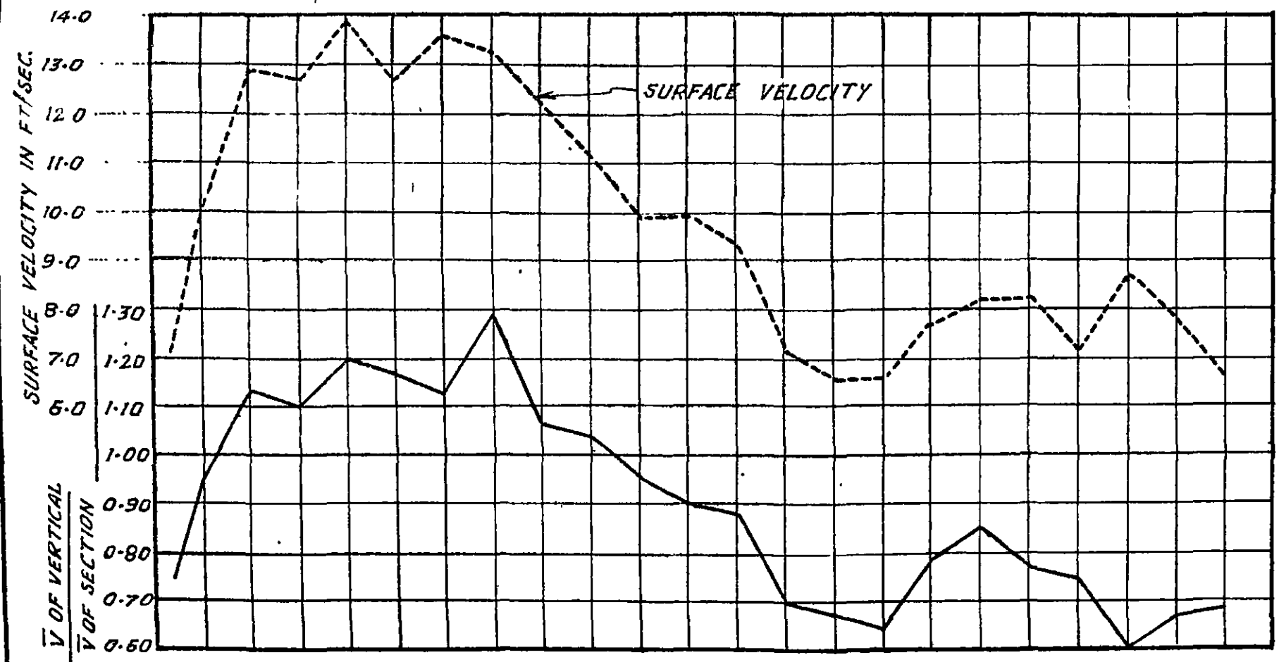
FIG. 3. MODEL OF RIVER GANGA MOKAMEH BRIDGE VELOCITY DISTRIBUTION CURVES BRIDGE ALIGNMENT CROSS SECTION WITH REPELLING SPUR 5000 FT. LONG. (2.5 MILES U/S OF BRIDGE SITE) MODEL SCALE - HOR. 1"=500', VER. 1"=67' DRAWING SCALE - HOR. 1"=1500', VER. 1"=30'
