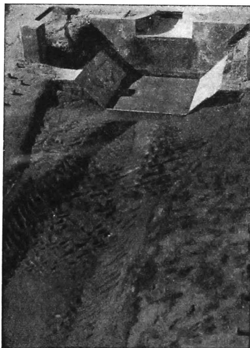
Photo No. 5543—Looking upstream, shows the scour pattern after a run of seven hours under conditions of flow depicted in Photo No. 5544. Notice the heavy deposit of eroded material formed by the movement of sand from the eroded sides towards the central portion.
