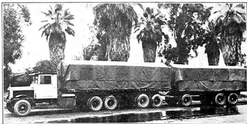
Figure 2.—A 6-wheeled tractor truck, a 4-wheeled semitrailer, and a 6-wheeled full trailer
