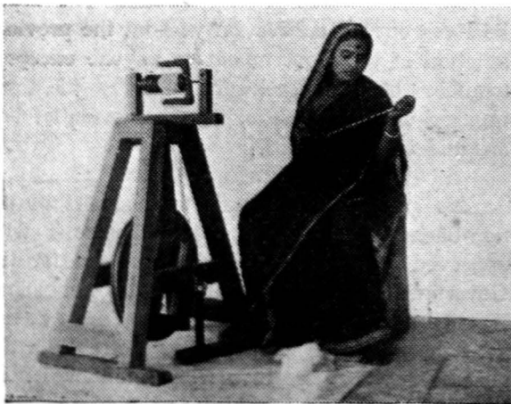
Spinning of wool with a Treadle Charkha at the Sheep Breeding Farm, Poona. (Carded wool may also be seen in the foreground).
