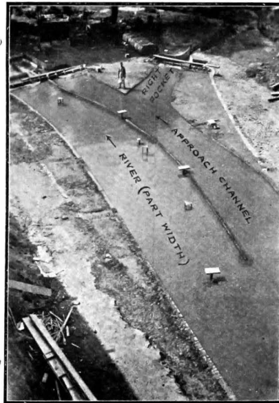
Photo 2061. Looking downstream. Series I Experiment 1 with the original design of lay-out, viz. length of sill 700 ft. with its top at R. L. 183.5. The banks upstream and downstream of the raised sill were vertical as originally proposed.
