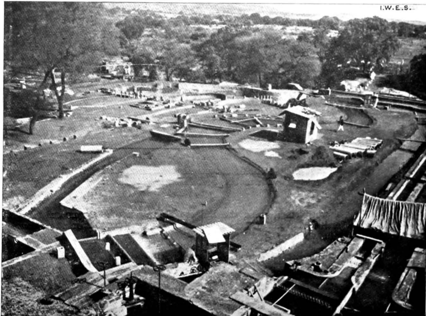
Photo H. 1458. Large-scale, short tidal model of Hooghly from Amaalpara to Ichapur, 15 miles north of Calcutta, where a "knuckle" has formed. Tides generated at both ends.
