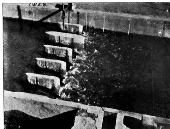
Photo 401. Same water levels as in Photo 440, with pavement lowered and slopes altered to 1 in 5 upstream and 1 in 10 downstream, sill raised to R. L. 177.
