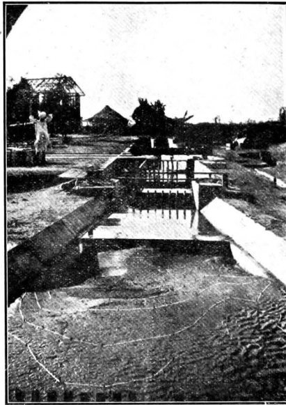
Photo 662. 1/24th scale model of Tando Mastikhan Fall with 1 in 10 diverging sides. F. S. Q \cong 10,590 cusecs. Fall \cong 8.7 ft. showing downstream scour, which would have caused failure of pavement.
