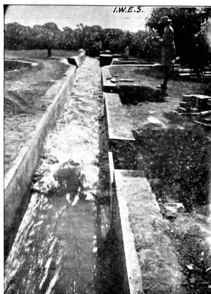
Photo 134. Two dimensional model of sill of Sukkur Barrage (as designed with pavement sloping at 1 in 70). Q \cong 420,000 cusecs. Sill at R. L. 176 and downstream water level at R. L. 184.2. Standing wave at downstream end of pavement which would have failed.
