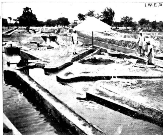
Photo 865. Experiment No. 4: 1 in 5 convergence upstream of the Mithrao and a long raised sill in front of the Mithrao and Khipro Canals. (Looking downstream).
