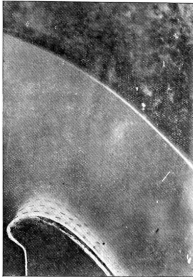
Photo 2255. Separation of boundary layer at crest of high coefficient weir, indicated by lifting of short silk threads, with formation of slight return roller near glass side wall due to side wall drag. Deflection of threads inwards denotes flow towards middle of sill where negative pressure unrelieved.
