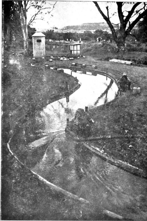
Photo H. 1467. Long tidal model of the Hooghly, showing tidal bore passing Palta, 12 miles north of Calcutta. Originally the model was >1,000 ft. long. Later reduced to 500 ft. with tidal generation at both ends.
