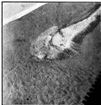
Photo 2125. Nose with elliptical sector and loose stone protection laid at 3:1 slope. Showing reduced damage after \approx 900,000 cusecs. (Q of Approach Channel \approx 30,000 cusecs.)
