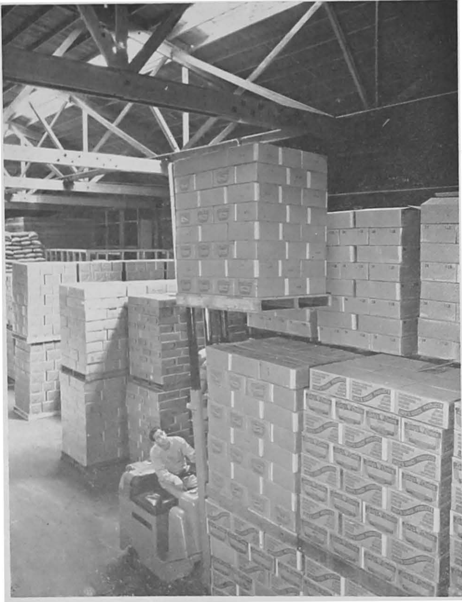
FIG. 40—Lift Truck and Palletized Storage
