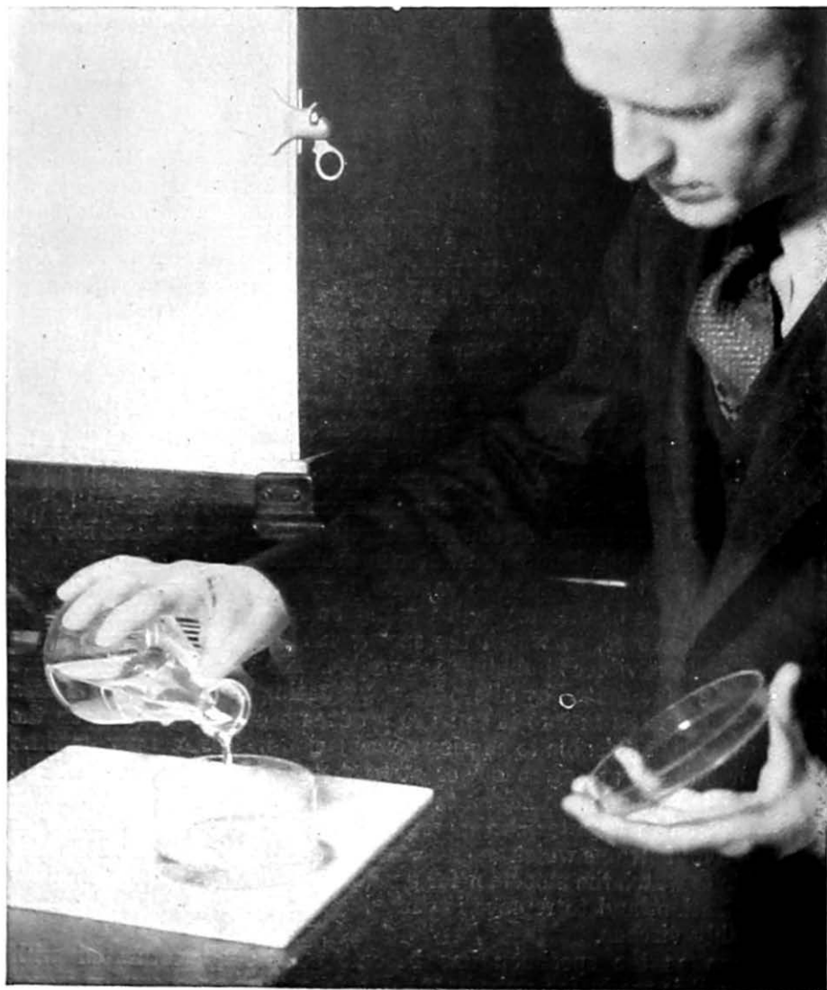
FIGURE 13.—A small amount of casting sirup is first poured into the mold and polymerized to serve as a supporting base for the specimen.
