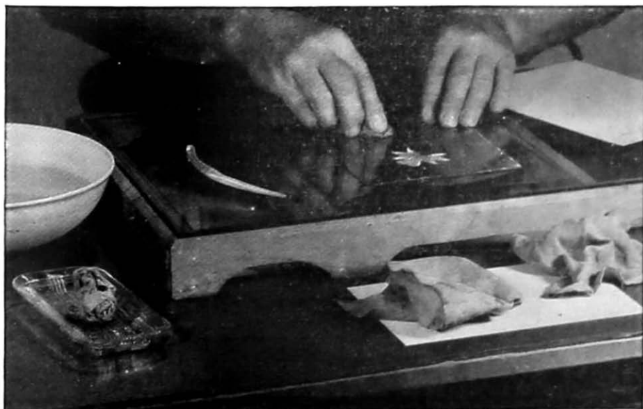
FIGURE 6.—After the temporary cover film has been removed the dried preservative is carefully washed from the plastic plate with paper toweling or chamois skin moistened with water.
