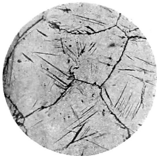
FIG. 10. Coarse grained tyre steel etched in Sodium Picrate. X 100
