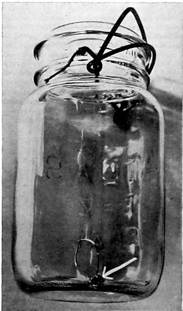
Figure 10. Jar Showing Stone and Break Caused by Temperature Shock.
