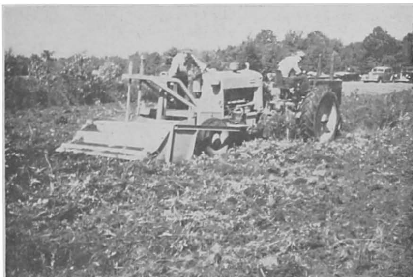
Figure 14. Bushes, Shrubs, and Weeds Are Chopped and Mixed with Soil by Rotary Tiller as First Step in Pasture Improvement.
