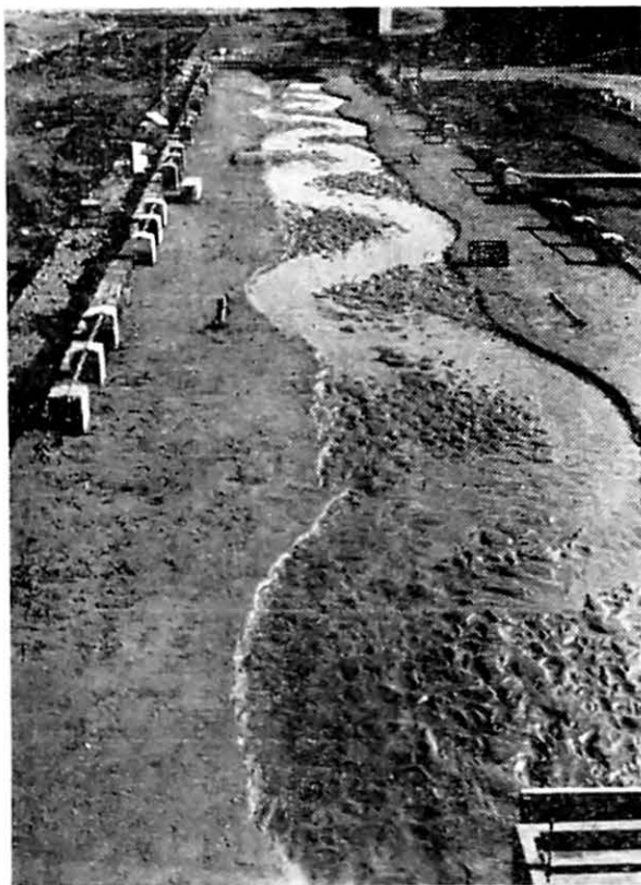
Figure 2 : Showing meanders developed in an experimental channel
