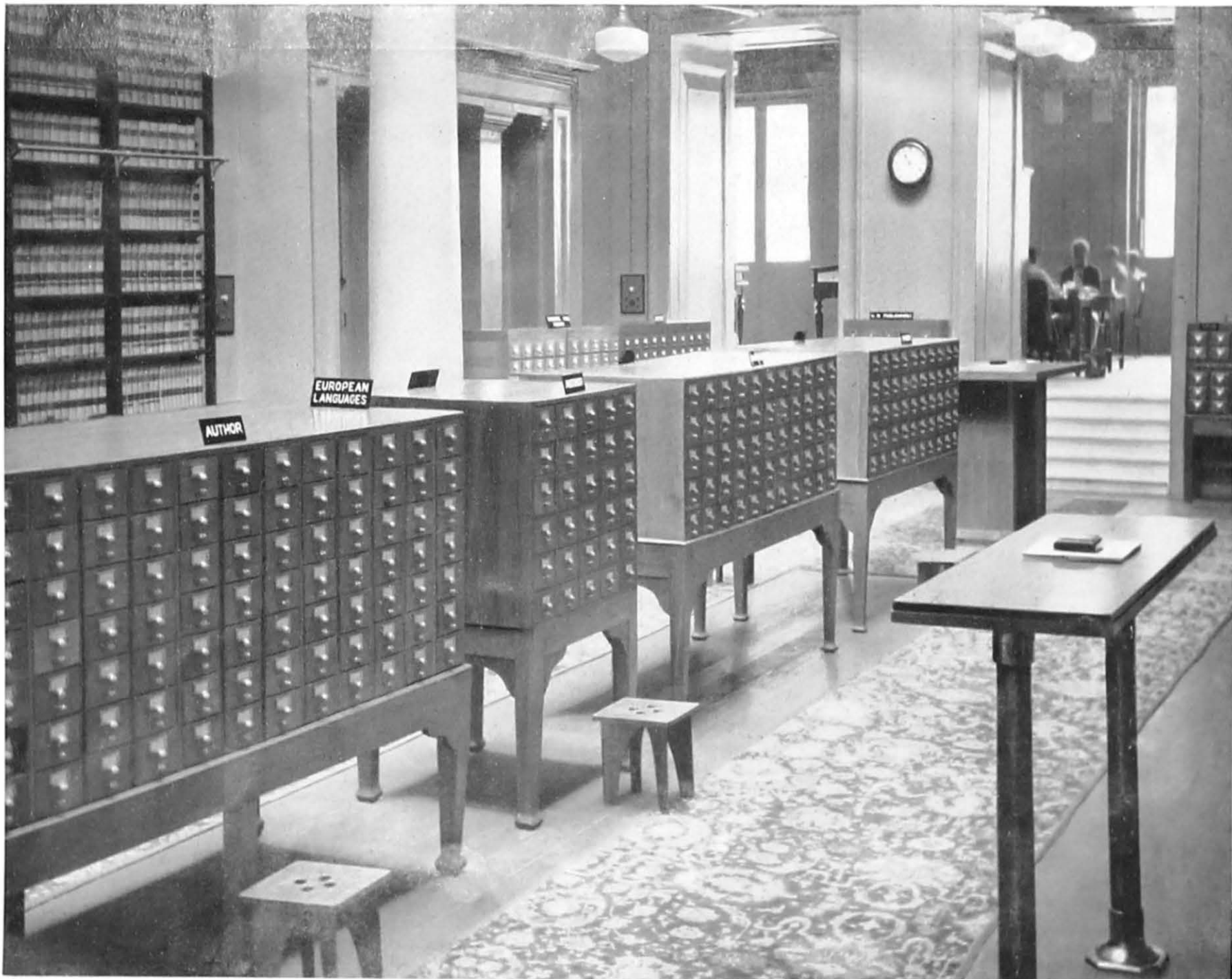
PLATE 3. A general view of the card cabinet room. The low stools and the tall tables make it easy for the reader to refer to the cards and note down his requisitions. The breaking up of the central mass redeems monotony and facilitates movement of readers from the "Author" side of the catalogue to the "Subject" side.
