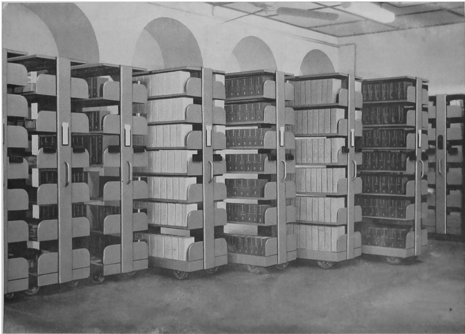
PLATE 9. The Chinese Collection in their characteristic box containers on the rolling-stacks. This picture very well illustrates the compactness, mobility and neatness of this method of shelving.
