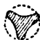
FIG. 27.—The transverse section of a short collapsed tube (after Fairbairn). The dotted line represents the original outline—the shaded area the form after collapse.
