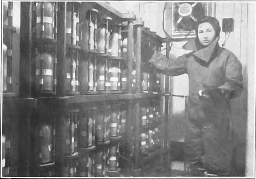
Vertical Spin-freezers in the Freezing Room of the Large Drying Plant.
