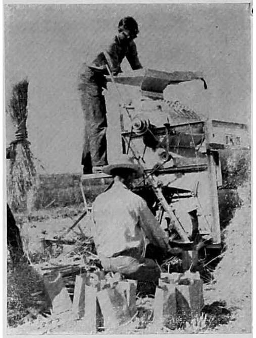
A nursery thresher built especially for measuring the yield of grain in an experimental row a rod long. The machine can be hitched to a car for hauling. It sets up in a minimum of time. A conversion table on the side tells directly how many bushels per acre the grain will rate—and it even weighs the sample of grain and gives the weight of that variety per bushel.
