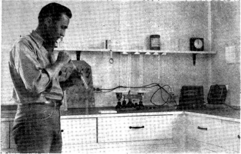
Soils technician tests one of many soil samples for nitrogen, phosphorus, potash, lime, acidity, soluble salt, and percolation
