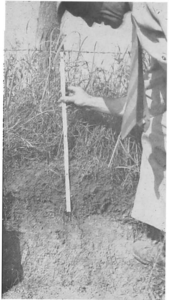
FIGURE 2. — The upper crust of the earth is the top soil. It usually has a "richer" color. This is the area from which the plant's roots take in a large amount of moisture and plant food. In this photograph the darker portion is the 7 inches of top soil. The subsoil lies underneath the top soil.
