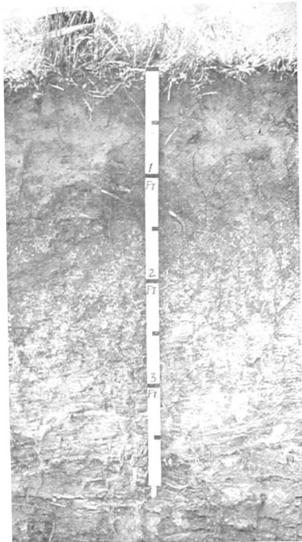
FIGURE 3. — This is a soil profile. The first foot is surface soil or top soil. The second and third feet are the subsoil. From the third foot down is parent material which is sandstone and shale.
