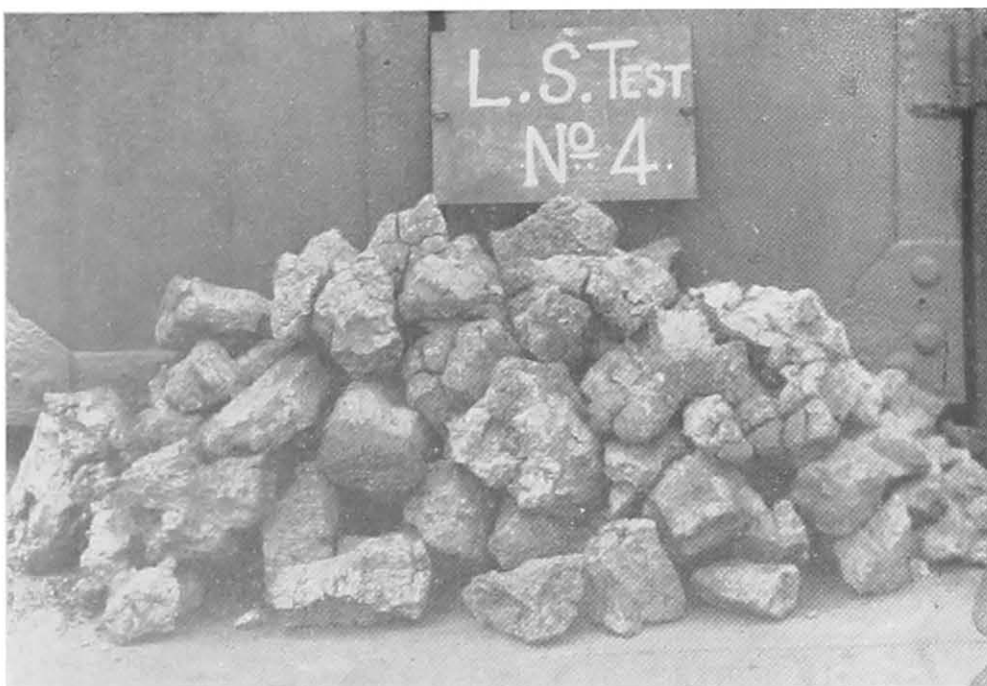
PLATE 1 -- NORMAL COKE FROM MIXED CHARGING COAL AS USED IN TATA'S COKE OVENS
