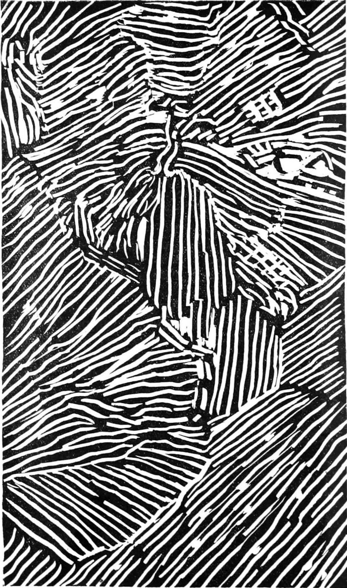
Fig. 54. This is a highly magnified picture (approximately 3000 times) of the surface of an ingot of iron. The pattern is made by the crystals of iron that formed within the ingot as it solidified. The crystals are very small and are all jumbled up with one another.
