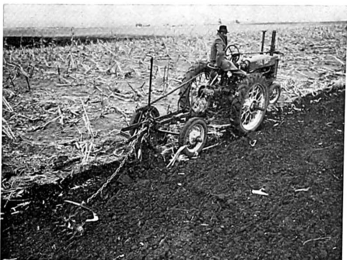
Fig. 5. Pneumatic tires on the tractor make pneumatic tires on field machines desirable. Used automobile tires will often serve satisfactorily. (Photo courtesy C. K. Shedd, Bur. of Agr. Engr., U. S. Dept. of Agr.).
