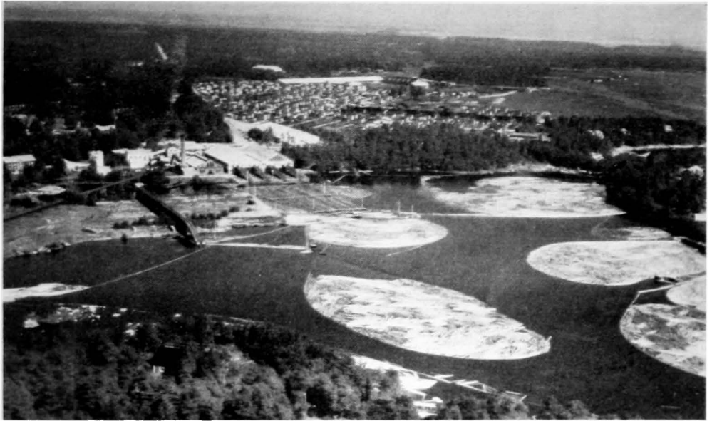
Sawmill at Ljusnan River. Millions of logs come floating to the mouths of the rivers where the sawmills are located.
