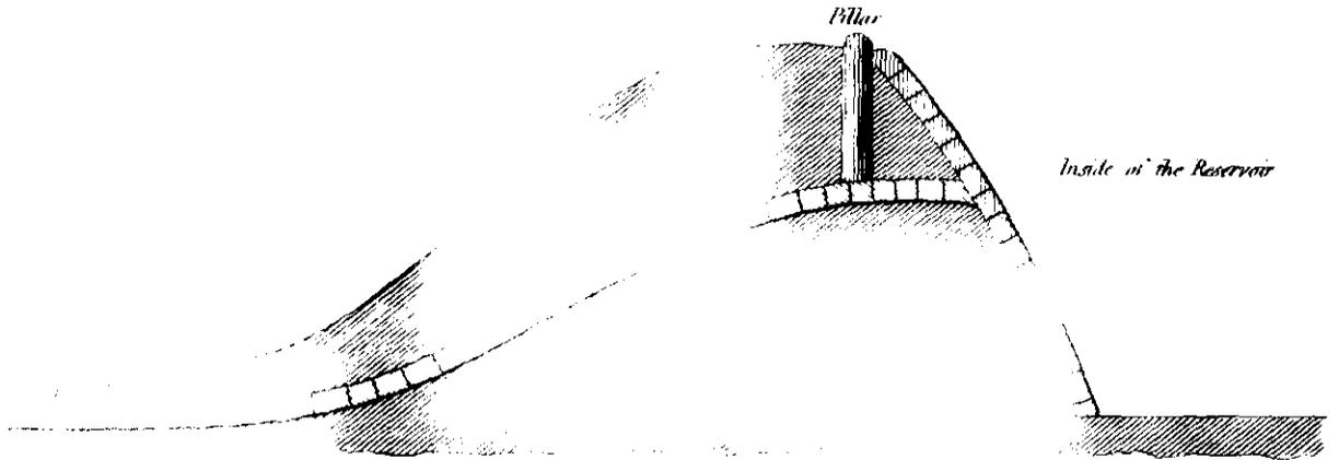
*Transverse section of the bank and shaft of an Eddy, or Race.*
