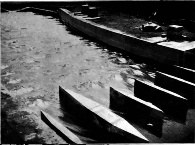
Pointed pier 1 in 5 upstream ; 1 in 10 downstream. (Looking downstream.) (I. D. R. N. 11.)
