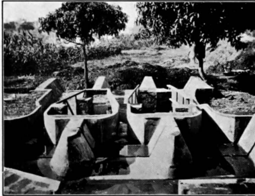
Small models of Flume Fall at Distributary No. 5, Mutha Right Bank Canal. (I. D. R. N. 26.)*
