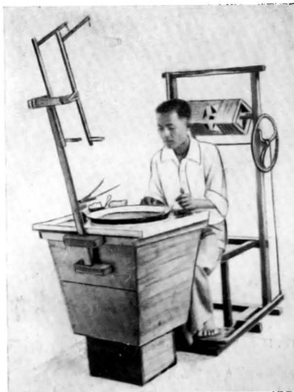
Fig. 16. Ashi-bumi or treadle reeling machine. The lower smaller box is simply a support to raise the even box.
