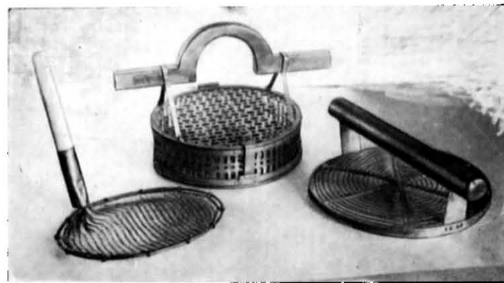
Fig. 51. Cocoon cooking utensils. Brass cage in the middle, its two circular covers are hinged and can be opened. Brass wire disc on the right hand side and stainer on the left.
