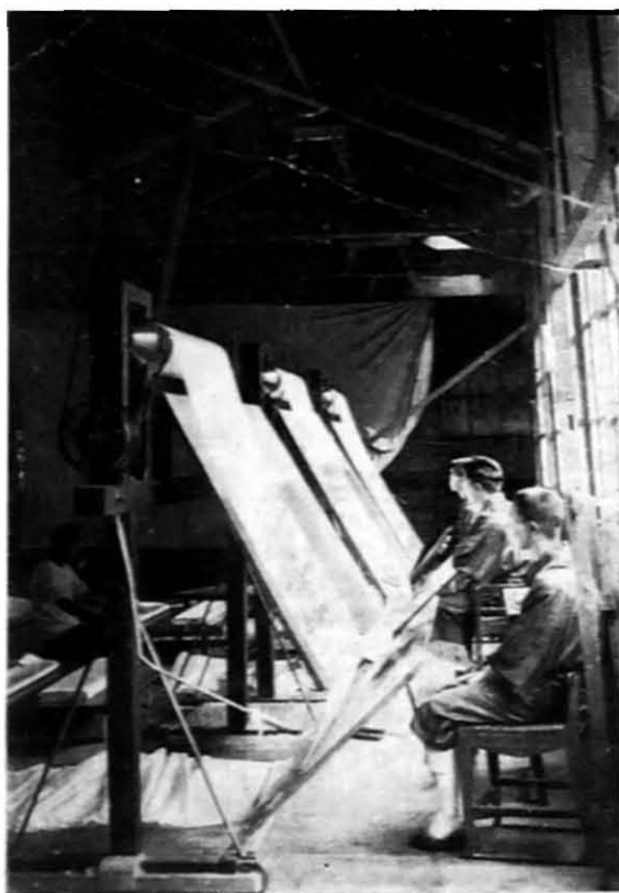
Fig. 54. General Inspection Stand (Fukui Inspection House).
