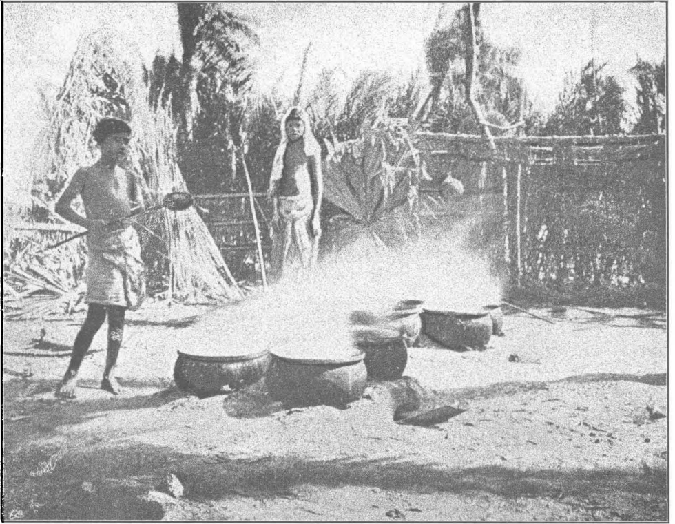
BENGAL FURNACE AND PANS FOR BOILING JUICE OF THE DATE PALM.
