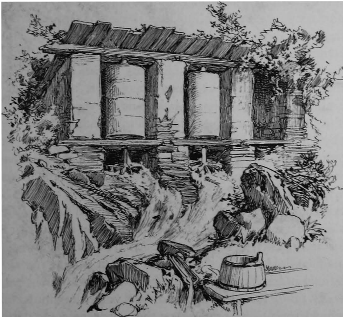
FIG. 2.—Praying-barrels propelled by water-wheels, at Soñum.
