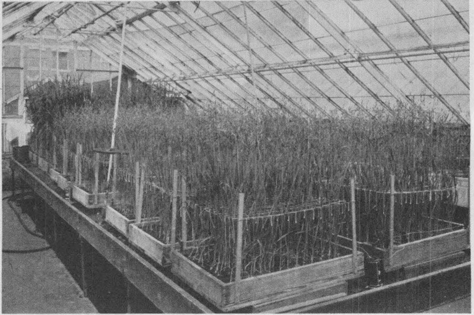
Fig. 5. Earth cell test with oats, 1932. Alternate flats are equipped with the copper-zinc electrode combination. Two lots have additional current supplied by a dry cell. The high fertility lots are at the far end of the bench.
