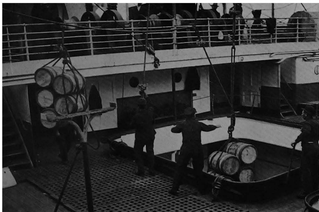
Two falls are being worked in this hatch. The winches for this hatch are on the deck above. The low coamings are dangerous
