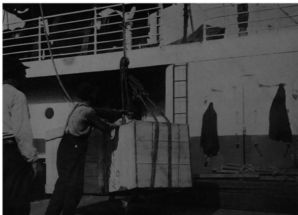
The gangway man unhooks the up and down fall from a swinging draft to which the burton fall has been attached. The draft will now be swung over the ship's side and landed on the pier
