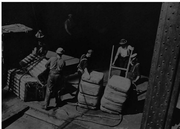
Drafts landed on the pier. Observe on the floor the rope sling from which the bags have just been removed
