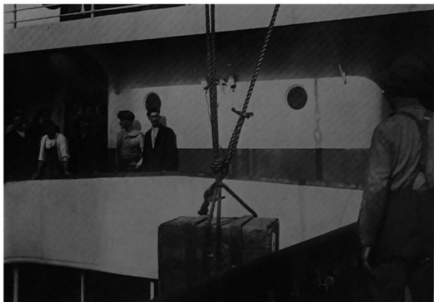
A rising draft showing the burton hook adjusted
