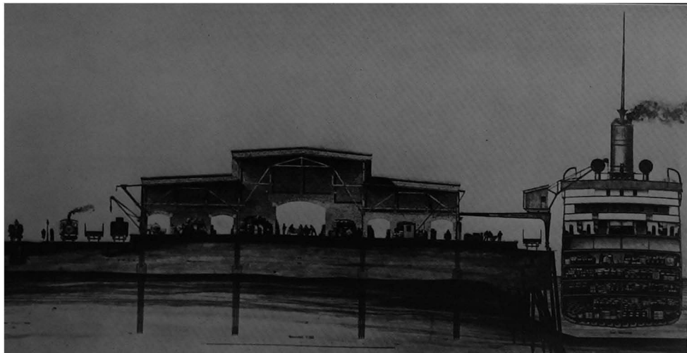
Cross section of the Crown Prince quay, Hamburg
