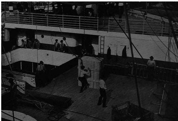
A large draft has been landed on deck. The gangway man is unhooking the up and down fall. As no regular place is provided for the men's coats, they are seen hanging and lying about
