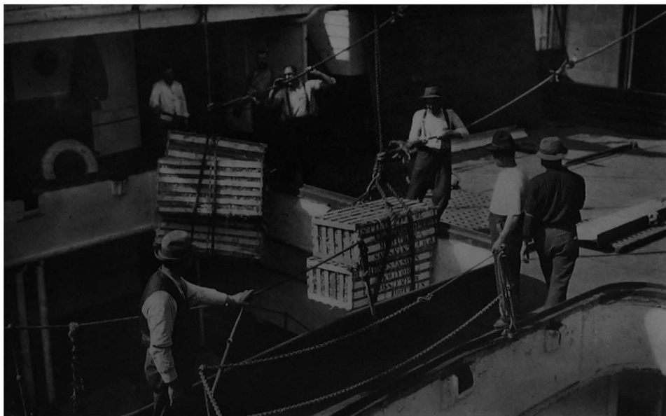
Two gangs are being worked in this hatch. Drafts have reached the hatch coamings at the same time and the hookers-on have just caught them with the hooks of the burton falls. The working of two falls in the same hatch is one of the things most dreaded by longshoremen
