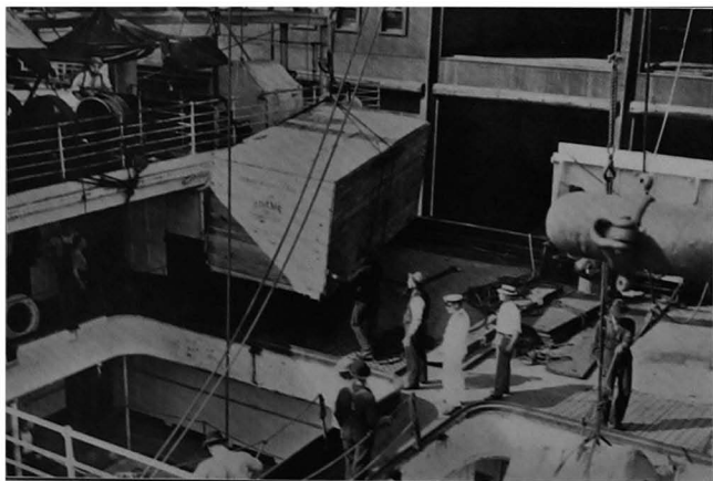
The boxed automobile as it swings athwart the ship on its way to be lowered to the pier. The gangway man steadies it with a touch of his hand. To the right is seen a draft just rising from an adjoining hatch. The hooker-on is in the act of catching it with the burton fall
