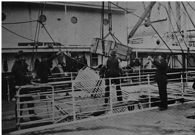
Deck men at work discharging cargo. Two drafts are coming out of this hatchway at the same time, involving danger to the men. One draft is made up of corrugated iron; the other is a "fruit box" (see p. 35)
