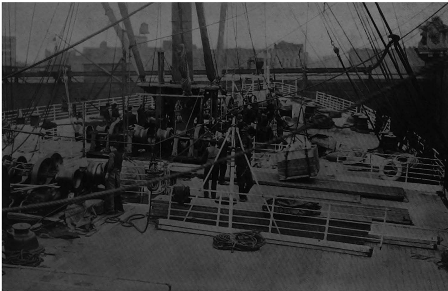
Discharging cargo from the forward hatches. In this picture the tangle of gear is shown. The winches for two hatchways can be seen, with the booms and mast necessary in handling cargo
