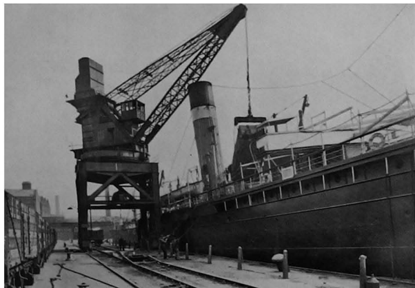
Hydraulic moveable coaling crane, Liverpool. Capacity thirty tons. The latest coaling device
