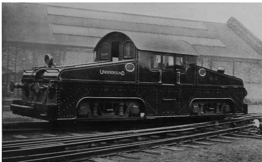
Electric Locomotive used on Central London Railway before adoption of the Multiple-Unit system.
