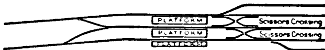
Arrangement of tracks, platforms, and cross-overs at above ground station used both for stopping and through trains.
