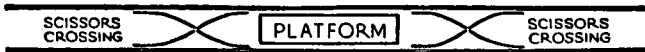
Track diagram of Liverpool Street station (underground) showing cross-over roads at each end.
