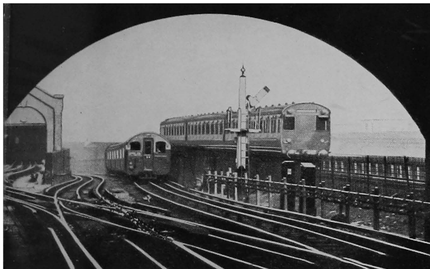
Side by side. Bakerloo and London, Midland, and Scottish trains near Queen's Park Station. Note the differences in size and the Upper Quadrant signal.
