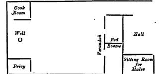
These houses, from being enclosed within walls, have no proper ventilation, and the rooms are so dark as sometimes to require a lamp, day and night.
