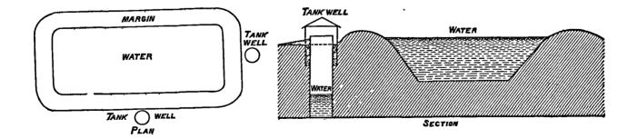
Wells sunk in clean ground at convenient places, and protected as already described, would sapply tank water naturally filtered, and probably there would be no objection to draw the water by iron buckets, chain and windlass in a mixed community.
