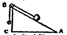
Inclined Plane (C A, base; C B, height; A B, inclined plane)
