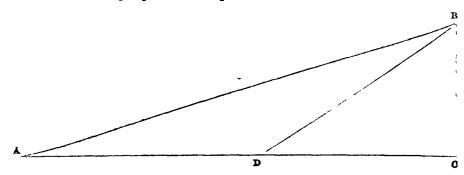
If A B represent a given gradient, it appears to me that, in the end, just as much power must be exerted to move a given load, say 100 tons, from one point to the other by any other disposition of the rails—as, for instance, A D, D B—as if the load had been moved along the uniform slope A B.
