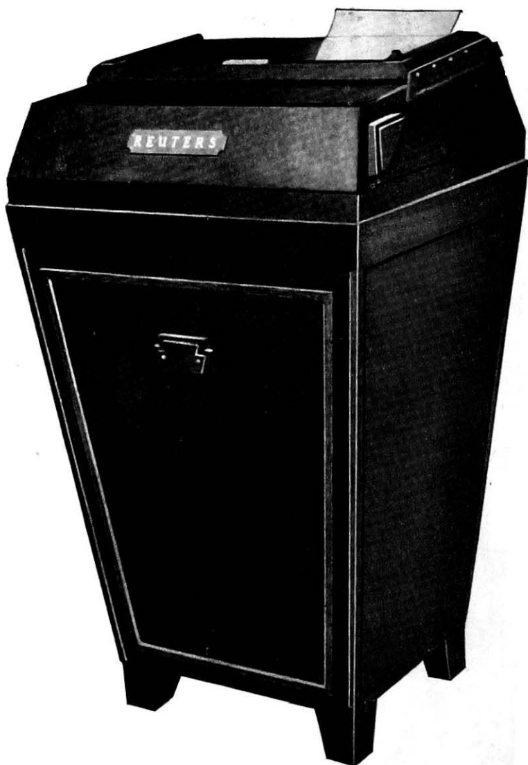
PLATE I.—THE CREED TELEPRINTER.
