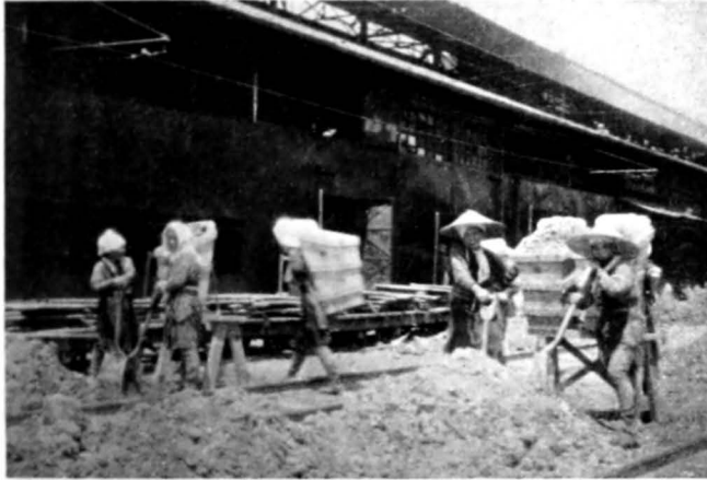
FIG. 101.—Women workers at the Ashio copper smelter transport clay for the furnace linings from a near-by hill.
