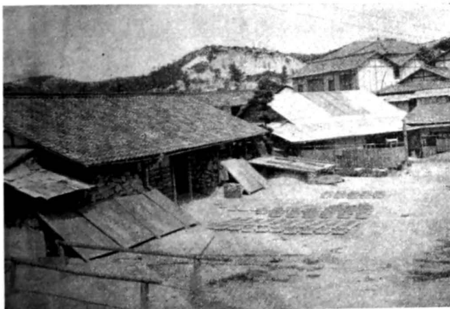
FIG. 60.—The potteries in Seto are small household establishments where most of the operations are done by hand. The ware is dried in the sun before it is fired. The kaolin deposit is in the background.
