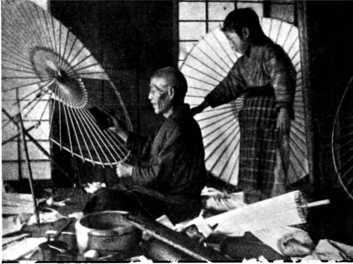
FIG. 68.—The Japanese umbrella is the product of a number of shops. In this one the paper is being attached to the ribs. (Photograph by H. Suito, Tokyo.)
