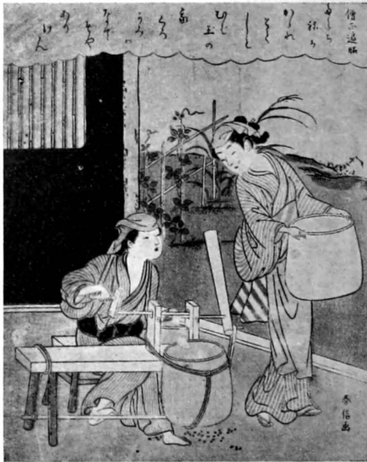
FIG. 26.—The seeds were removed from the raw cotton by passing it between wooden rollers. (From an early eighteenth century print by Harunobu in the collection of the Metropolitan Museum of Art.)
