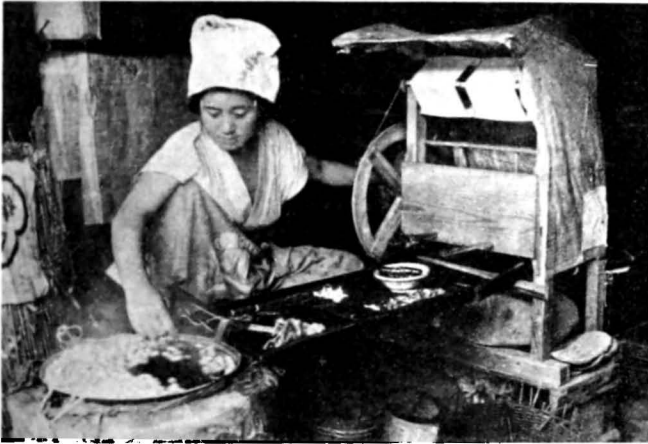
FIG. 36.—The primitive hand reel of feudal Japan is still used in the homes of the farmers for the production of raw silk. (Photograph by H. Suito, Tokyo.)
