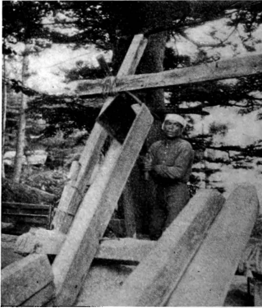
FIG. 91.—The primitive method of cutting planks still common in Japan. This photograph was taken in a wood yard on Lake Chuzenji in 1926. Compare Figures 25 and 92.
