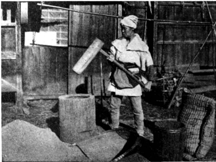
FIG. 18.—Rice was husked in small establishments with primitive wooden mortar and pestle. (Photograph by H. Suilo, Tokyo.)
