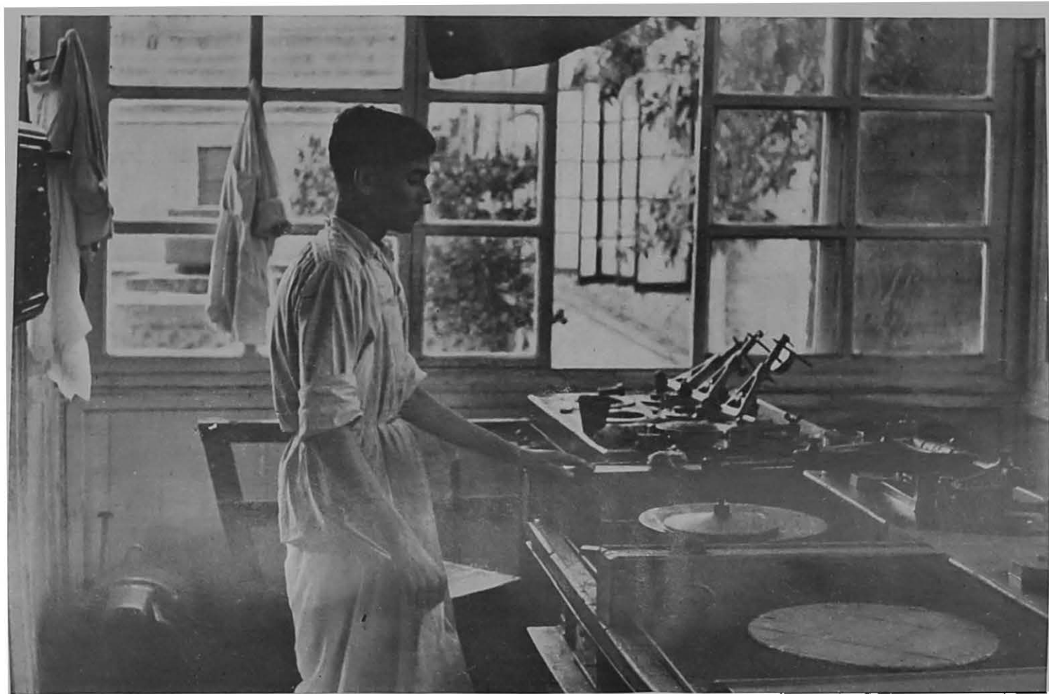
POLISHING MIRRORS IN THE MATHEMATICAL INSTRUMENT OFFICE.
