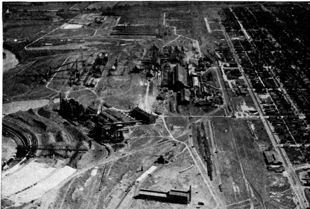
FIG. 400.—Layout of a large iron and steel plant (National Tube Company) in Lorain, Ohio. Piles of coal, iron ore, and limestone are conspicuous along the waterway in the left foreground. ( Photograph by Somogy-Lorens. )
