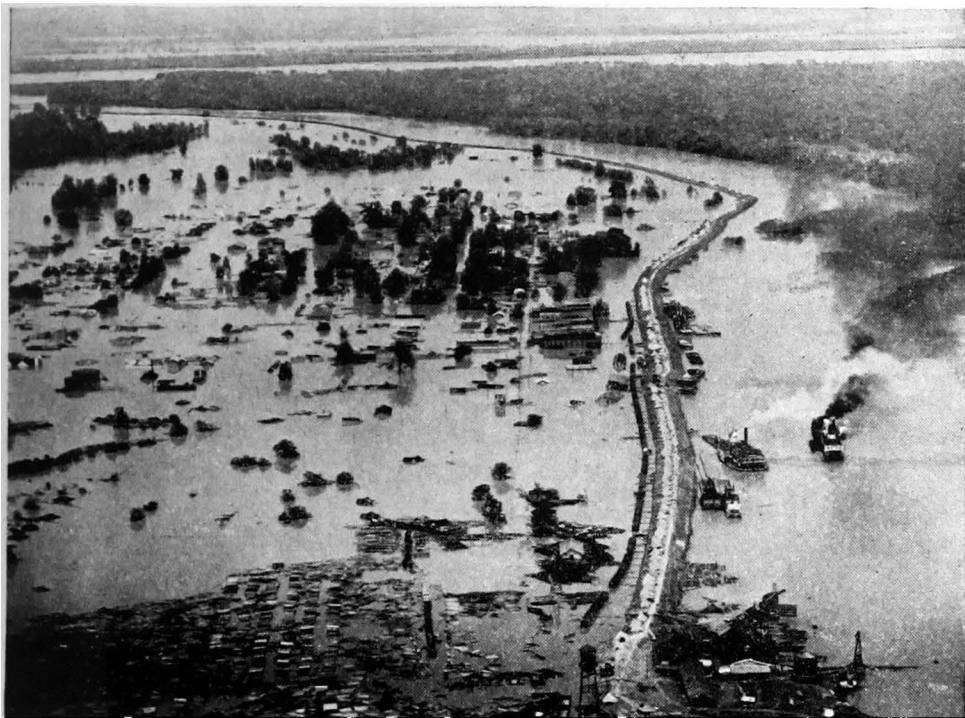
FIG. 160.—High water on the lower Mississippi floodplain. The artificial levee is the only land remaining unsubmerged. The main channel of the river is seen in the far distance. The locations of several natural levees associated with minor channels are indicated by the belts of submerged woodlands and the town. ( Official Photograph, U. S. Army Air Corps. )
