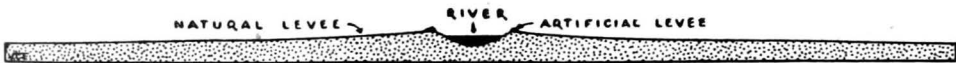
FIG. 158.—A diagram to show the transverse profiles of natural and artificial levees. Vertical scale considerably exaggerated.
