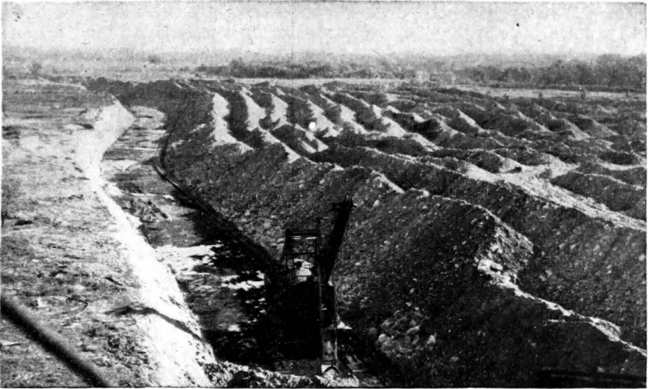
FIG. 327.—Giant furrows turned by power shovels in the process of strip mining in southern Illinois. The 4 ft.-thick bed of coal exposed in the bottom of the deep trench is mined out before the next furrow is turned.
