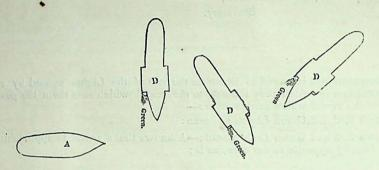
If A sees a White Mast-head Light above the Green Light, A knows that the vessel is a steam vessel, and is either approaching her in the same direction as B, or is crossing to starboard in some direction, as DDD.
