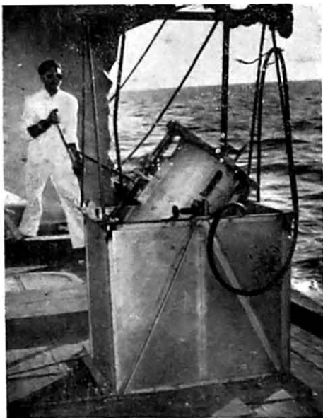
Photo 7 Injector being shaken for mixing its contents.
