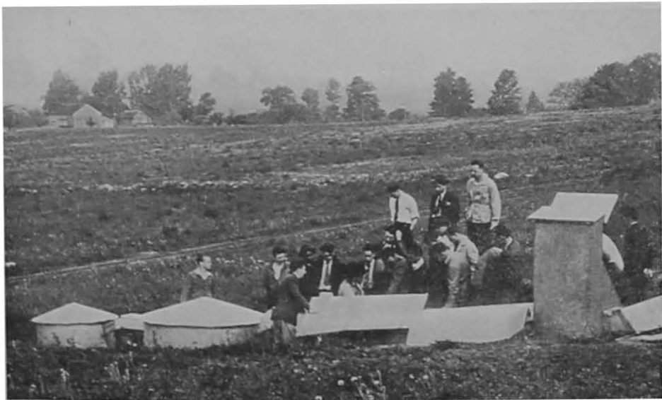
FIGURE 5. CATCHMENT TANKS FOR WATER AND SOIL FROM PLOTS SIMILAR TO THOSE SHOWN IN FIGURE 2
