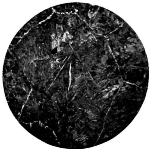
FIG. 11. Extremely coarse grained tyre steel etched in Nital. X 100
