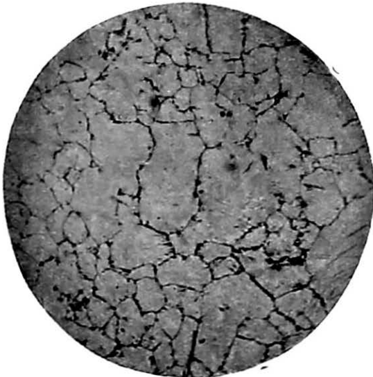
FIG. 20. Fine grained Axle steel etched in Sodium Picrate.
