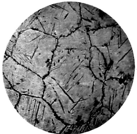
FIG. 21. Coarse grained Axle steel etched in Sodium Picrate.
