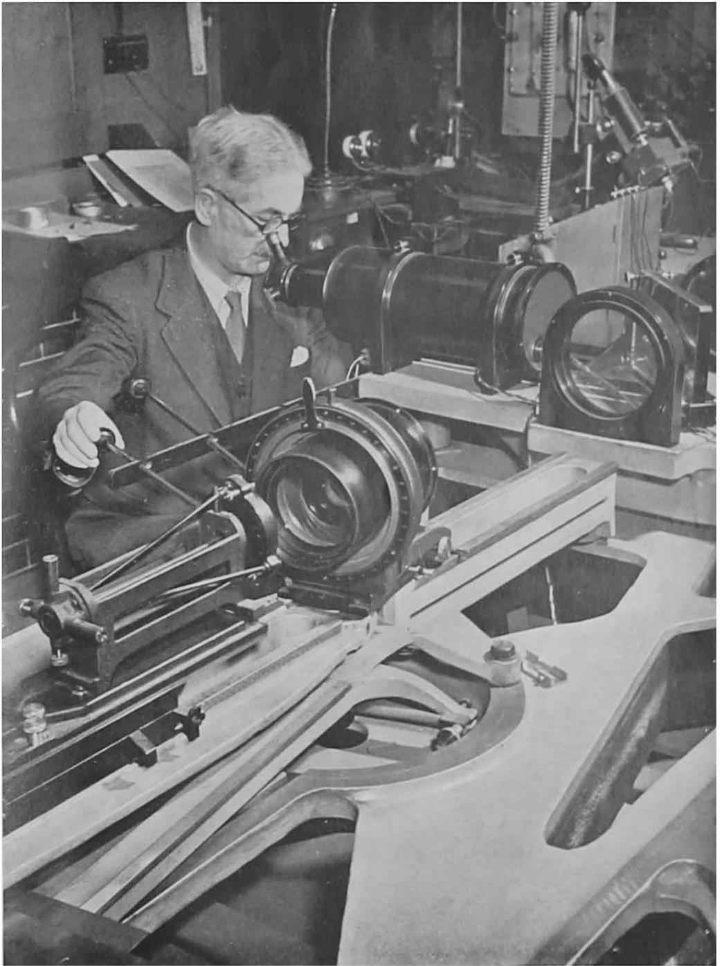
View of the observing portion of the ' Universal ' lens testing interferometer with an aerial camera lens under examination to obtain, in the laboratory, an estimate of the performance of the lens
