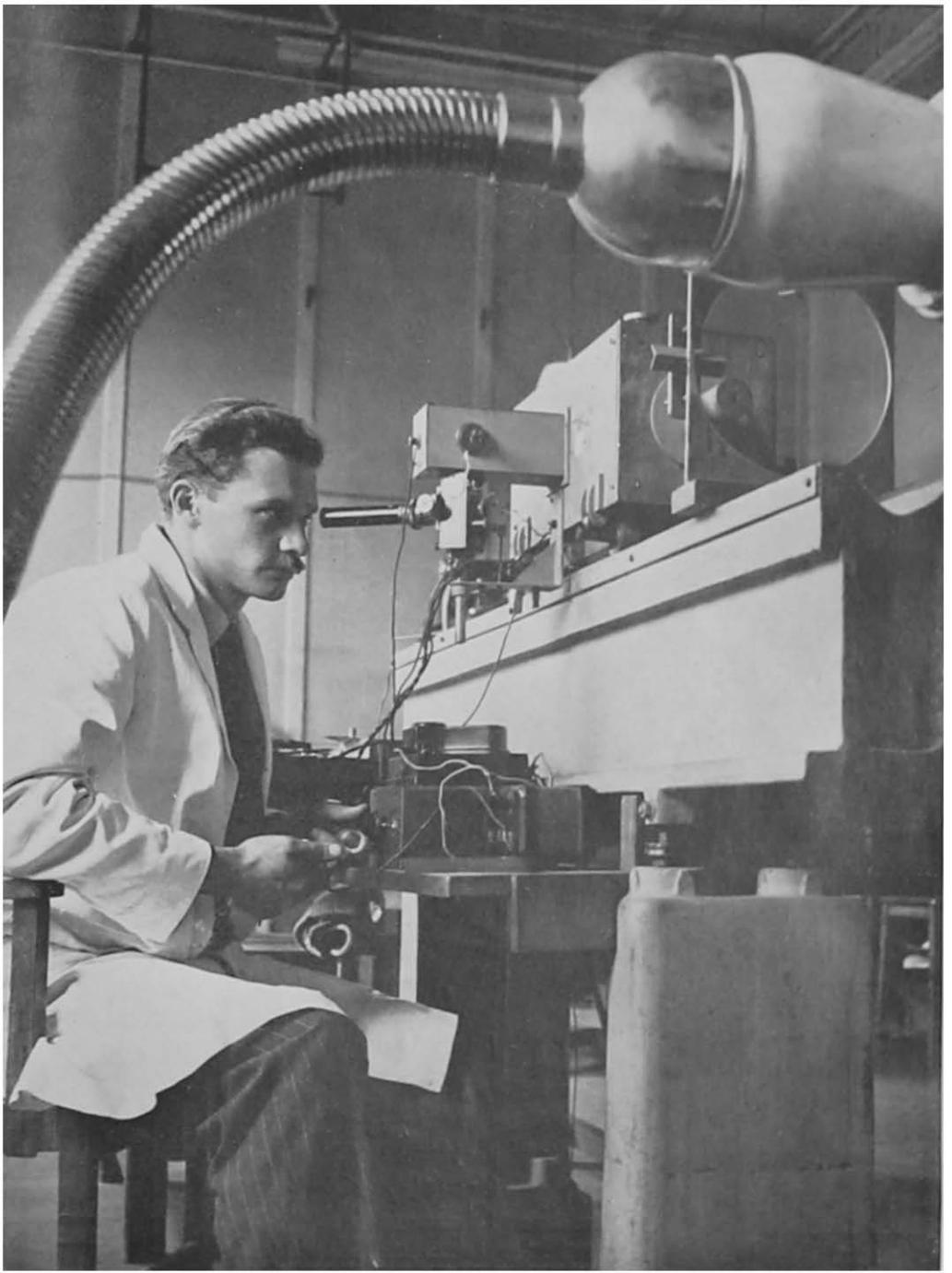
**This special apparatus is used by the Physics Division for the precise determination of X-ray intensities. Problems of protection against radiation are also the concern of this section**
