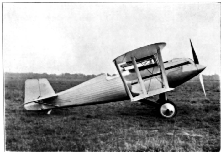
A HIGH-SPEED WATER-COOLED ENGINEED SINGLE-SEATER FIGHTER. THE FAIREY FIREFLY—430 h.p. Fairey Felix 12 Cylinder Vee Water-Cooled Engine.
