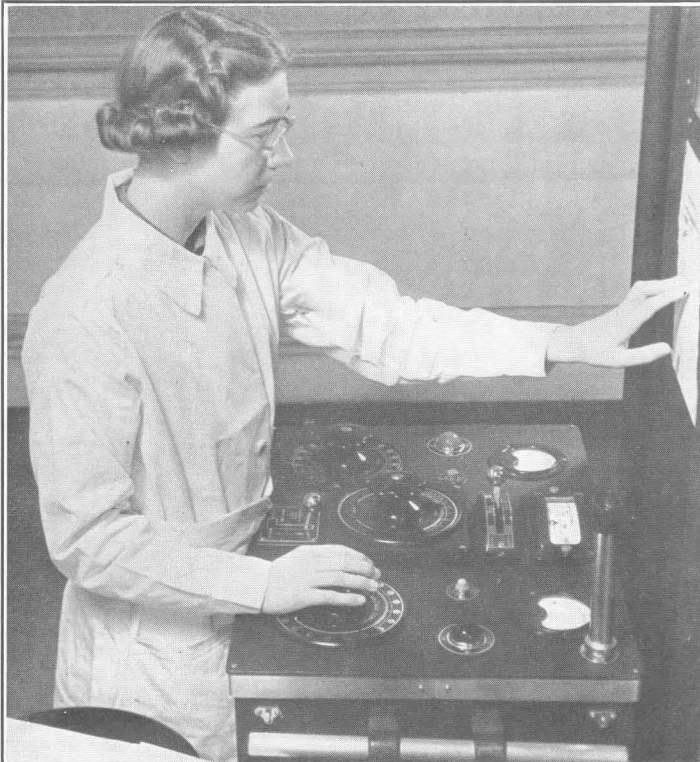
FIG. 5.—Threading the camera. Note tension control knob on right (see p. 20). FIG. 6.—Adjusting exposure conditions according to chest thickness measurement, by reference to the exposure table (see p. 21).
