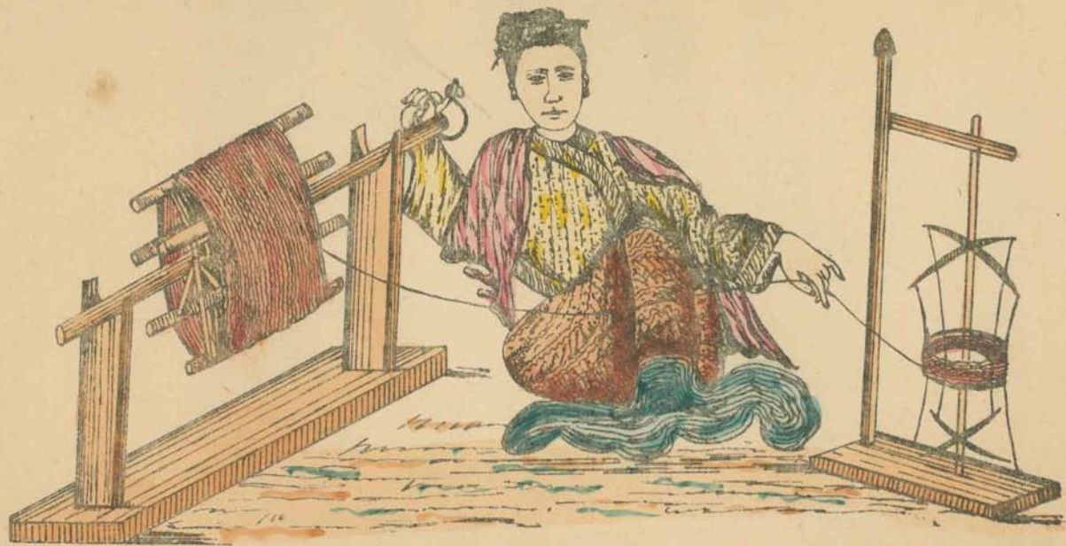
FIGURE XXVI.—Showing the process of transferring the small coils of Singapore silk thread ( shabekchi ) from Figure I to Figure II.
