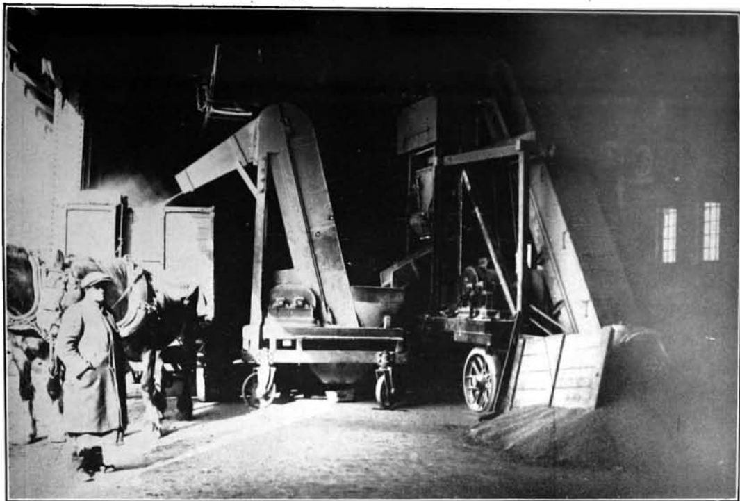
FIG. 18.—Bulk grain being weighed and loaded to horse wagon in dock transit shed, Glasgow.
