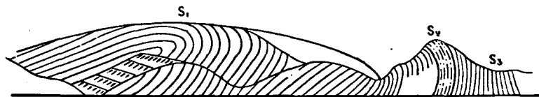
Fig. 8. Section of the south-eastern flank of the anticline of the Zelenetsky mountain: S 3 —light-coloured shales; S 2 —marls of the Middle Sarmatian stage; S 1 —dark-coloured of the Lower Sarmatian stage (after Andrusov).
