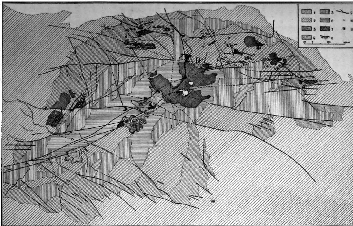
Fig. 14. Geological map of Nefte-Dag (after K. Kalitsky): 1—Ancient Caspian sediments; 2—the Baku stage; 3—the middle division of the Apsheronian stage; 4—alluvium; 5—clay with ferruginous laminae; 6—gray marl with Adelina voluta (4—6 belong to the lower division of the Apsheronian stage); 7)—covers of kir; 8 — outcrops of the oil-bearing strata; 9—faults; 10—hand-dug wells; 11—drill holes. I—IV—oil regions.
